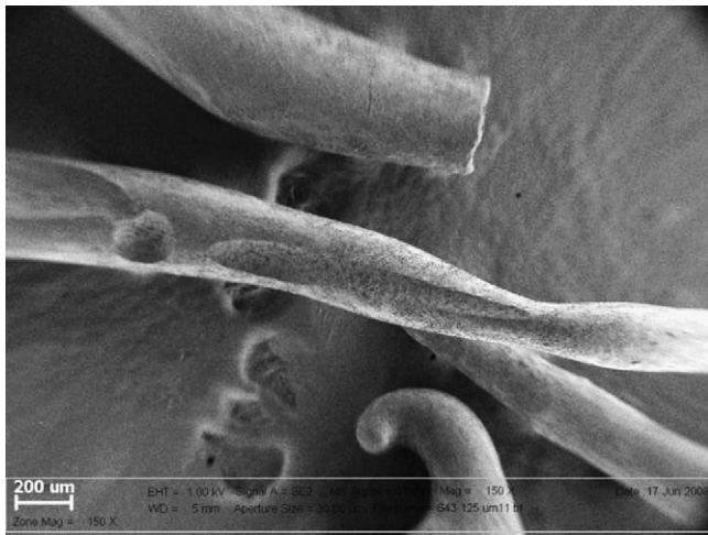
Fig. 3. Worm-like or needle-like particles produced at unsatisfactorily low atomizing pressure (at 1.050 bar).
